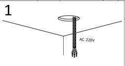
Thread the wire through the mounting hole.
