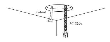
Open the mounting hole on ceiling according to the cutout size, and pass the wires through the hole.
