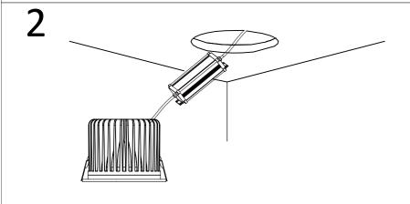
Cord according to the wiring instruction marked on the driver, and do the insulation protection well. And insert the driver into cutout on the ceiling.
