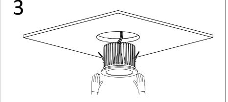
Press the mounting spring into the cutout in the ceiling and push the luminaire in.
