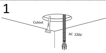
Open the mounting hole on ceiling according to the cutout size, and pass the wires through the hole.
