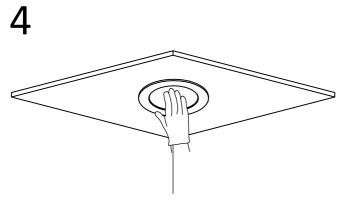
The installation is completed until the frame is flat with the ceiling. Adjustable downlight series can adjust the irradiation angle according to the demand to meet the lighting requirements.
