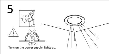
Warning: The fitting should be never covered by insulation gasket or similar materials under any circumstance. Please ensure that the wires are conneced correctly before turning on the power supply. Do not look emitting lights directly to avoid burning your eyes.
