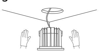
Press the mounting spring into the cutout in the ceiling and push the luminaire in.
