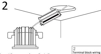
Connect the power cord according to the wiring instruction marked on the driver, and do the insulation protection well. And insert the driver into cutout on the ceiling.
